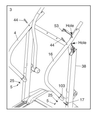
4. Attach the ground wire to the small hole in the side of the Right Handrail (16) with a Silver Ground Screw (99).
